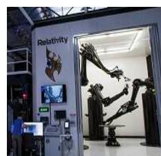
With its large 3D-printing machines, the startup claims that its rockets will require 100 times fewer parts than traditional rockets. "We'll only be experts in like two or three (technological) processes," he said, compared to traditional manufacturing with complex supply chains. "It's far easier."
