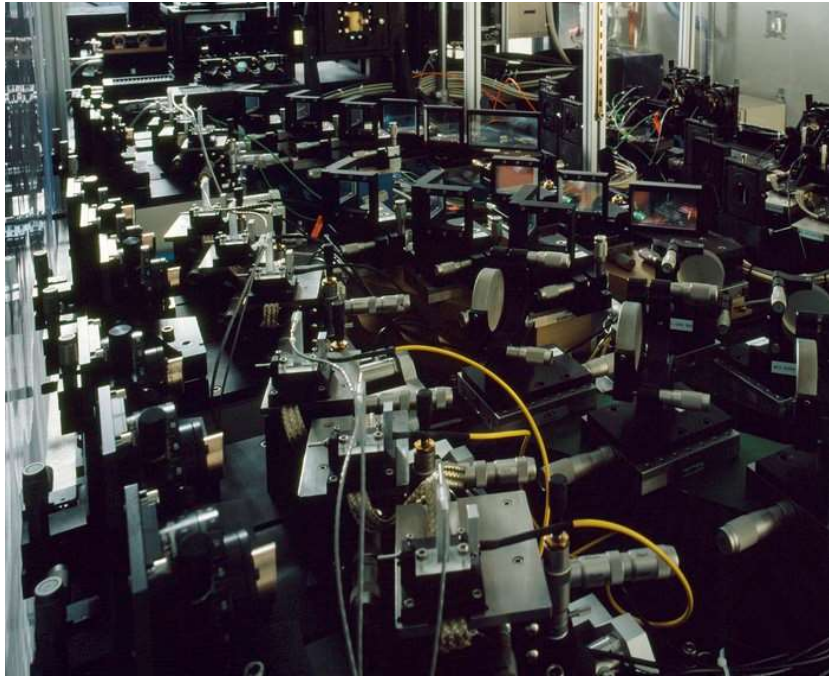
Beam combination at the AMBER instrument, VLT
