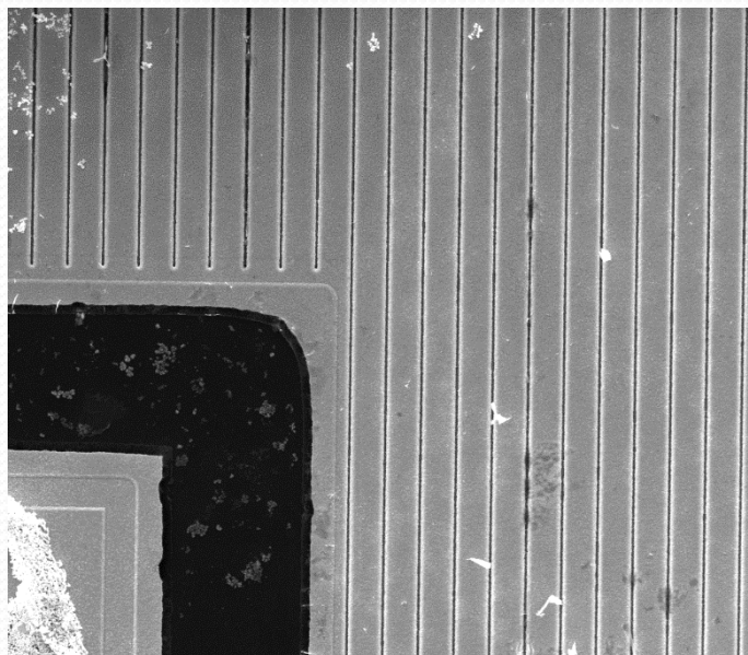
Exemple of multiple finger MOSFET
