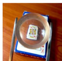
This is because FDM printers don't create 100% solid parts, partly for material usage reasons and partly for technical limitations. Even when setting the infill to 100%, there will usually be slight voids and gaps between the lines of plastic extrusion that inhibit the passage of light. It's likely that these 3D prints are also stronger due to their homogeneous molecular structures, which is its own totally separate benefit to printing 100% solid parts. .
