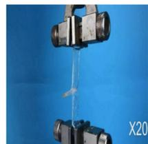
A new type of adhesive designed by the scientists from the Harvard John A. Paulson School of Engineering and Applied Sciences (SEAS) and Xi'an Jiaotong University in China can strongly adhere wet materials—such as living tissue and hydrogel—and be easily detached using a specific frequency of light. The adhesive consists of an aqueous solution of polymer chains spread between two, non-sticky materials—similar to jam between two slices of bread.
