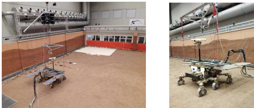
Figure 21: GTM Rover model in ALTEC facilities (image credit ESA/TAS-I/ALTEC)
