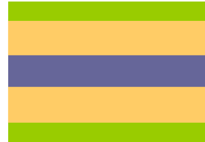
Deposition of \text{Si}_3\text{N}_4 film(800nm) by LPCVD*
