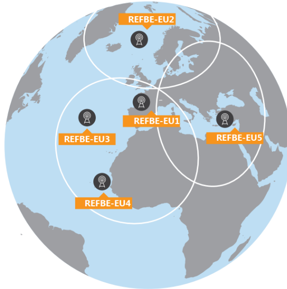
Fig. 2. SAR/Galileo Reference Beacons (REFBE) distribution over the European Coverage Area (ECA)
